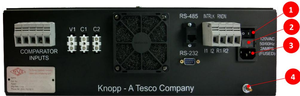
Figure 2.4. KATC-V2 Main Power Supply
