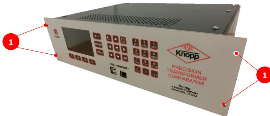
The instrument contains four mounting holes, ① as shown above, on the front panel and should be mounted to the KVTS where the previous comparator was placed. All four screws can then be mounted as they were prior through the four mounting holes. If not in a KVTS, mount as normal into a 3U enclosure.
