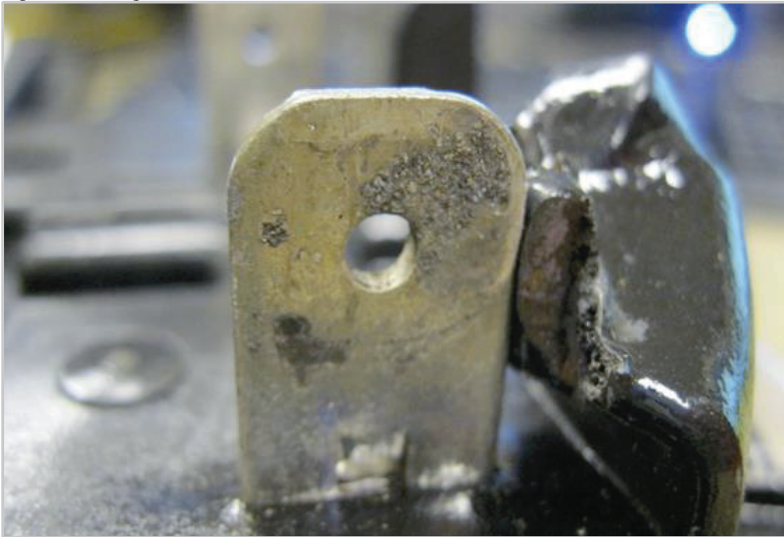
Figure 1. Pitting and Discoloration of a Hot Socket Meter Blade Returned from the Field
