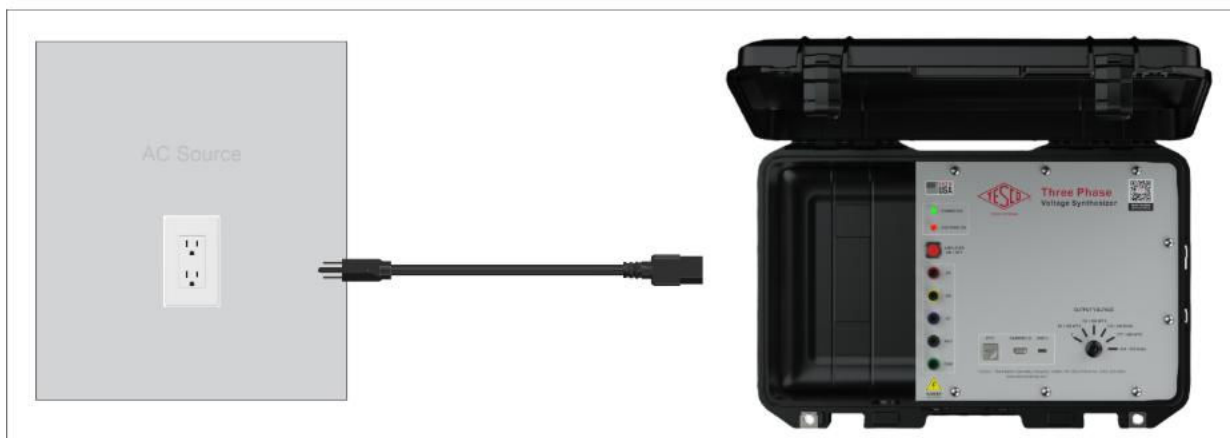
Figure 2.4.1 Power the 6440 unit at the meter shop using a 120VAC / 240VAC source using a standard power cord (Nema 5-15 plug). The supplied cord is about 10 feet long (3 meters)
