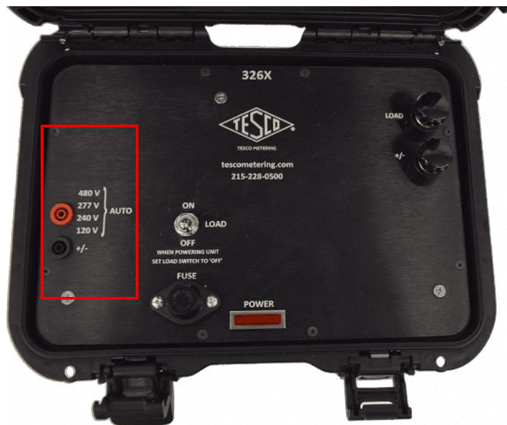
Figure 2.5.1 Voltage Input Connections on the unit.
