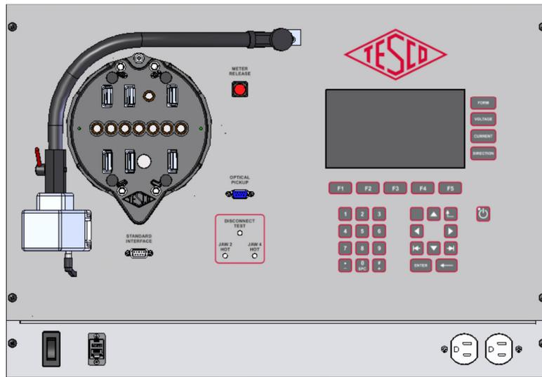
**Figure 4.1 - TESCO NextGen front panel**
