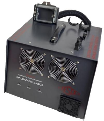
The PL4000 is an AC programmable load box that can test AC EV chargers up to 14kW. The unit is used with a T4000 or T4350. The load box works with single-phase AC charger (CCS1 / J1772 and NACS).
