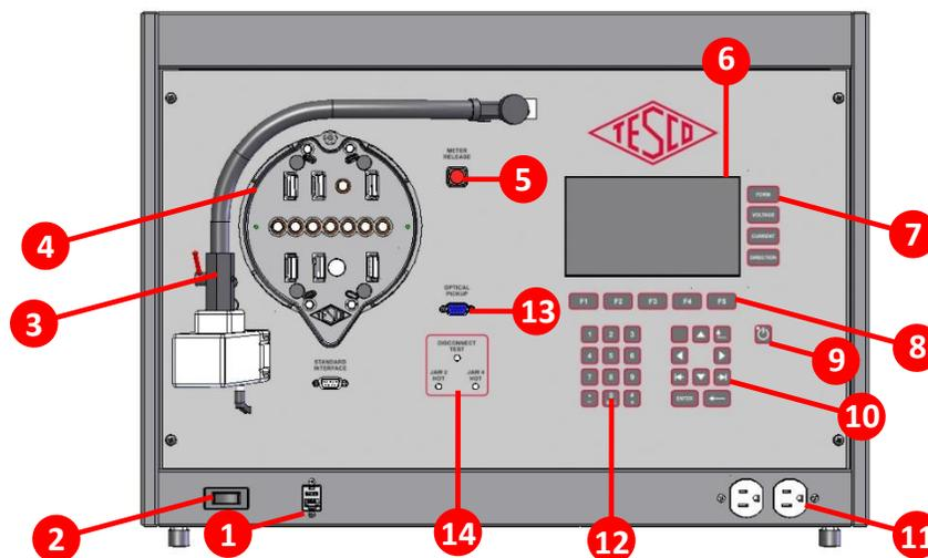
Figure 3.2.1a MTS-3050 Front Panel
