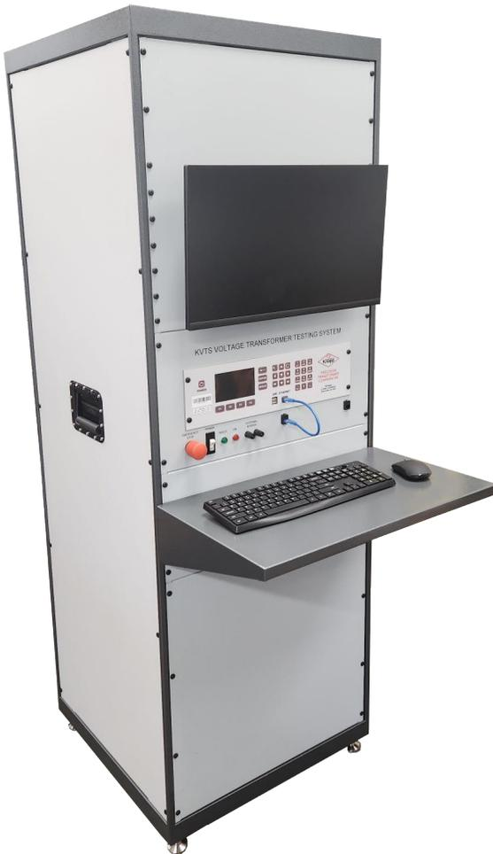
The Knopp Automated Voltage Transformer Testing System designed to measure the accuracy of instrument transformers having 120-volt secondary's and up to 48,000-volt primaries. The new automated KVTS-A enables increased stability of measurement and includes the control console which contains the control circuitry, digital ANSI standard burdens for increased accuracy, and the Upgraded Knopp Automatic Transformer Comparator.
