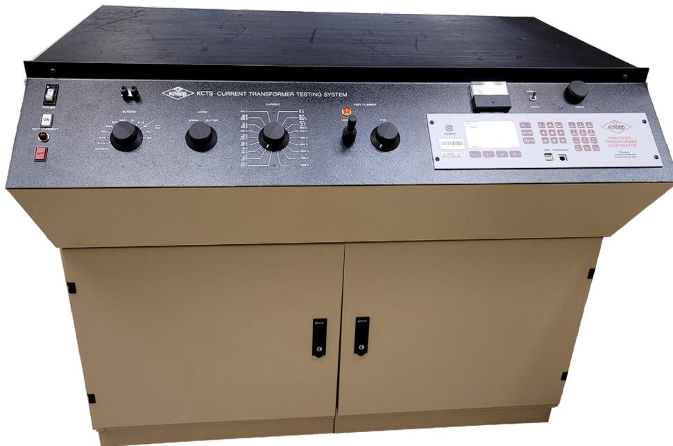
The Knopp Current Transformer Testing System (Type KCTS-8000) is designed to measure the accuracy of instrument transformers having 1 or 5 ampere secondaries and primaries of up to 8000 amperes. The system uses a high accuracy multi-range current transformer as a reference standard. All ANSI standard burdens are included. The phase angle and ratio errors of the transformer-under-test (TUT) are measured by the
