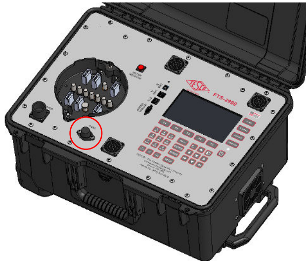
Figure 5.2a FTS-2990 Fuse Location
