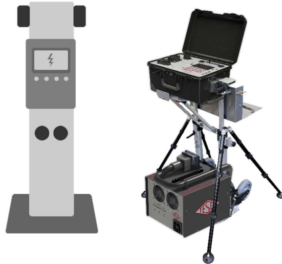
Figure 2.3b Suggested Vertical Oriented Setup with the PL4000. This application does not apply to the PL4150.
