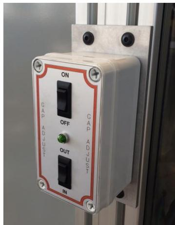
*Figure 7 – Rocker switch enclosure that controls gap adjustment*
