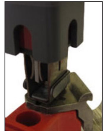
Red indication of a "bad" socket gap/loss of spring
