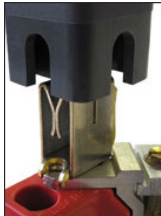
No indication of a "bad" socket gap/loss of spring force.
