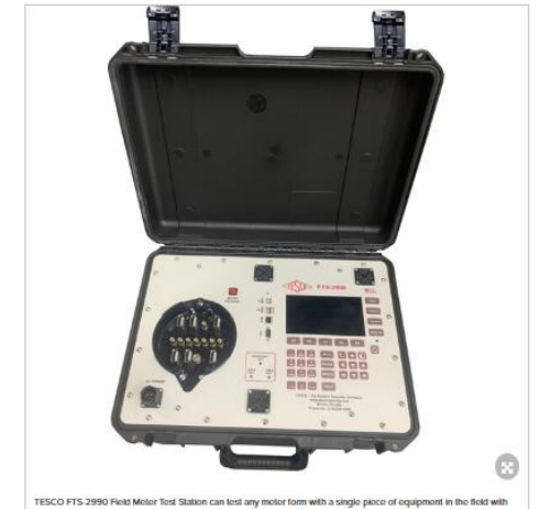
TESCO FTS-2990 Field Test Station can test any meter form with a single piece of equipment in the field with
