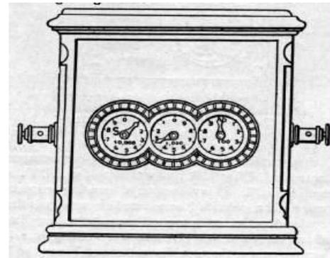
Image from original 1872 patent for Samuel Gardiner's electric meter and a rendering of the front cover
