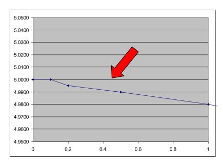
At 0.5Ohms of Burden the secondary current is still at 4.990A – Less than 0.3% change – Good CT!
