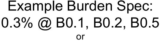
There should be less than the 0.3% change in secondary current from initial ("0" burden) reading, when up to 0.50hms of burden is applied
