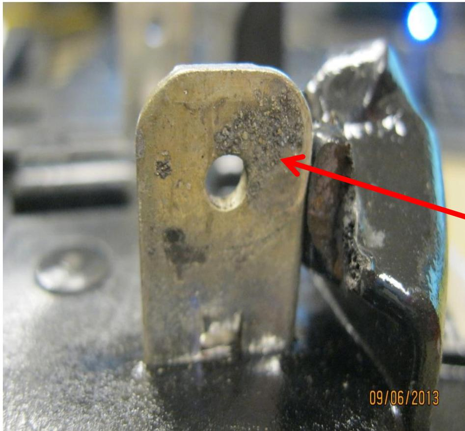
Jaws with intermittent connections will arc to the meter blade resulting in pitting on the blade.
