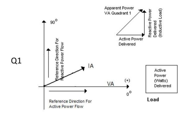
If you set up the calculation to Ignore received KWH(Q2 or Q3) as well as ignore any leading KVRH (Q4) then the above billing determinant can be honored.
