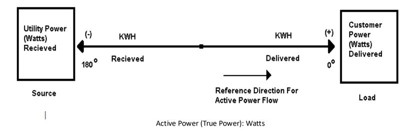
When the Active Power (Watts) flow from the "SOURCE" through the metering point and into the "LOAD" we say the Active Power (Watts) are being DELIVERED. Therefore, when the Active Power is being supplied by the "SOURCE" into the load it will be referred to as Delivered Power (Watts) and has a positive sign. **Standard billing determinants would be Delivered kW/kWh.**
