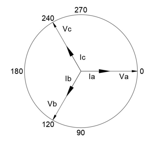
Phasor Diagram for 3-element, 4-wire Wye connected service
