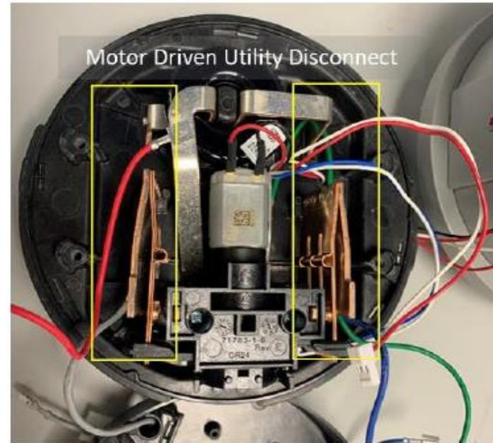
Figure 1. Utility disconnect switch and the generator relay
