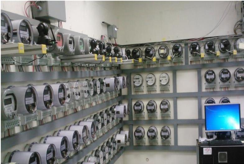
How well is a meter type performing in the field? Walk through the meter farm. That is a pretty good initial indicator.
