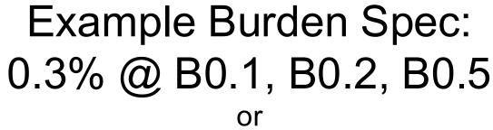
There should be less than the 0.3% change in secondary current from initial ("0" burden) reading, when up to 0.50hms of burden is applied
