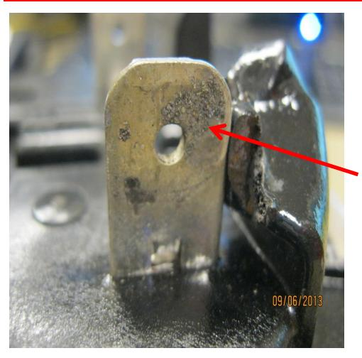
Jaws with intermittent connections will arc to the meter blade resulting in pitting on the blade.
