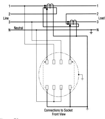
Three-Phase Four-Wire Wye With Two Equal-Ratio CTs
