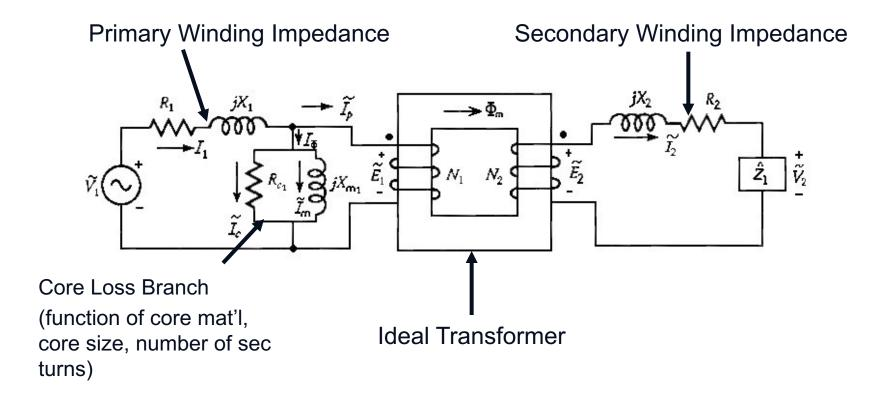
This is an illustration that the excitation current is the current lost from the primary current that does not get to the meter. Accuracy is largely a function of minimizing this excitation current and why transformer accuracy is typically negative.
