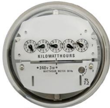
Old Electromechanical Meter
