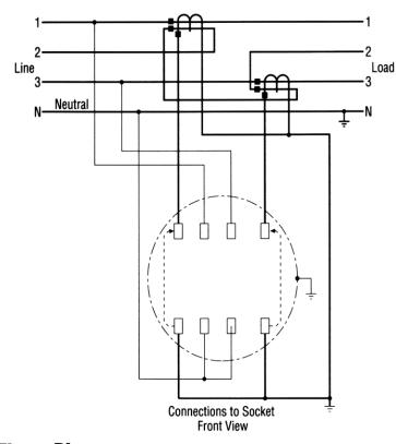
Three-Phase Four-Wire Wye With Two Equal-Ratio CTs
