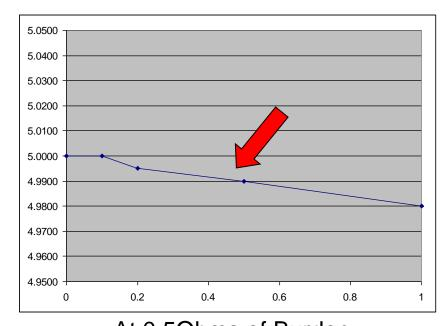
At 0.5Ohms of Burden the secondary current is still at 4.990A – Less than 0.3% change – Good CT! Initial Reading = 5Amps
