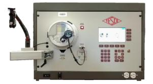
or by removing the meter and testing in a piece of field equipment or van mounted equipment with a meter socket for testing where the meter can be tested and returned to the customers socket in a minimum amount of time and without ever leaving the premises other than to return to the utility van.
