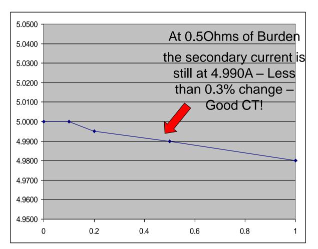
Initial Reading = 5Amps  $0.3\% \times 5A = 0.015A$  5A - 0.015 = 4.985A
