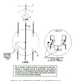
2 Stator, 3ø, 3 W (Network) Meter, Self-Contained
