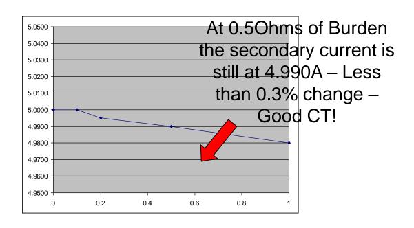
Initial Reading = 5Amps  $0.3\% \times 5A = 0.015A$  5A - 0.015 = 4.985A
