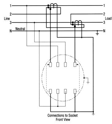
Three-Phase Four-Wire Wye With Two Equal-Ratio CTs
