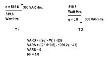
VA =  $\sqrt{(Watts^2 + VARS^2)}$ VA =  $\sqrt{(1039.2^2 + 0^2)}$ VA = 1039.2 Slide 42
