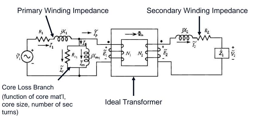
This is an illustration that the excitation current is the current lost from the primary current that does not get to the meter. Accuracy is largely a function of minimizing this excitation current and why transformer accuracy is typically negative.
