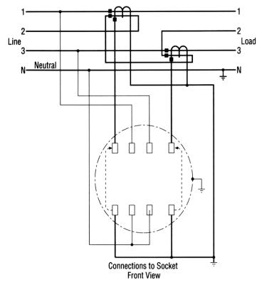
Three-Phase Four-Wire Wye With Two Equal-Ratio CTs
