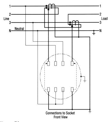
Three-Phase Four-Wire Wye With Two Equal-Ratio CTs
