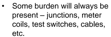
CT's must be able to maintain an accurate ratio with burden on the secondary.
