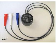
in time of the different voltage peaks of a multiphase supply. In addition, the Knopp Sequence Indicator enables one to make continuity tests. It is a valuable instrument in diverse fields involving polyphaser power apparatus, being employed by line and installation crews for public utility systems and industrial-plant electrical departments. It is, furthermore, helpful in the testing departments of public utility systems for laboratory and field testing.
