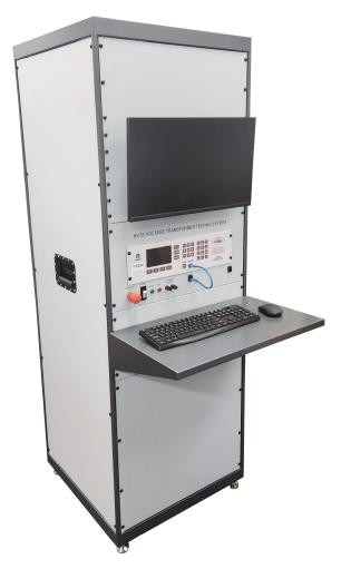
The Knopp Automated Voltage Transformer Testing System designed to measure the accuracy of instrument transformers having 120-volt secondary's and up to 48,000-volt primaries. The new automated KVTS-A enables increased stability of measurement and includes the control console which contains the control circuitry, digital ANSI standard burdens for increased accuracy, and the Upgraded Knopp Automatic Transformer Comparator.
