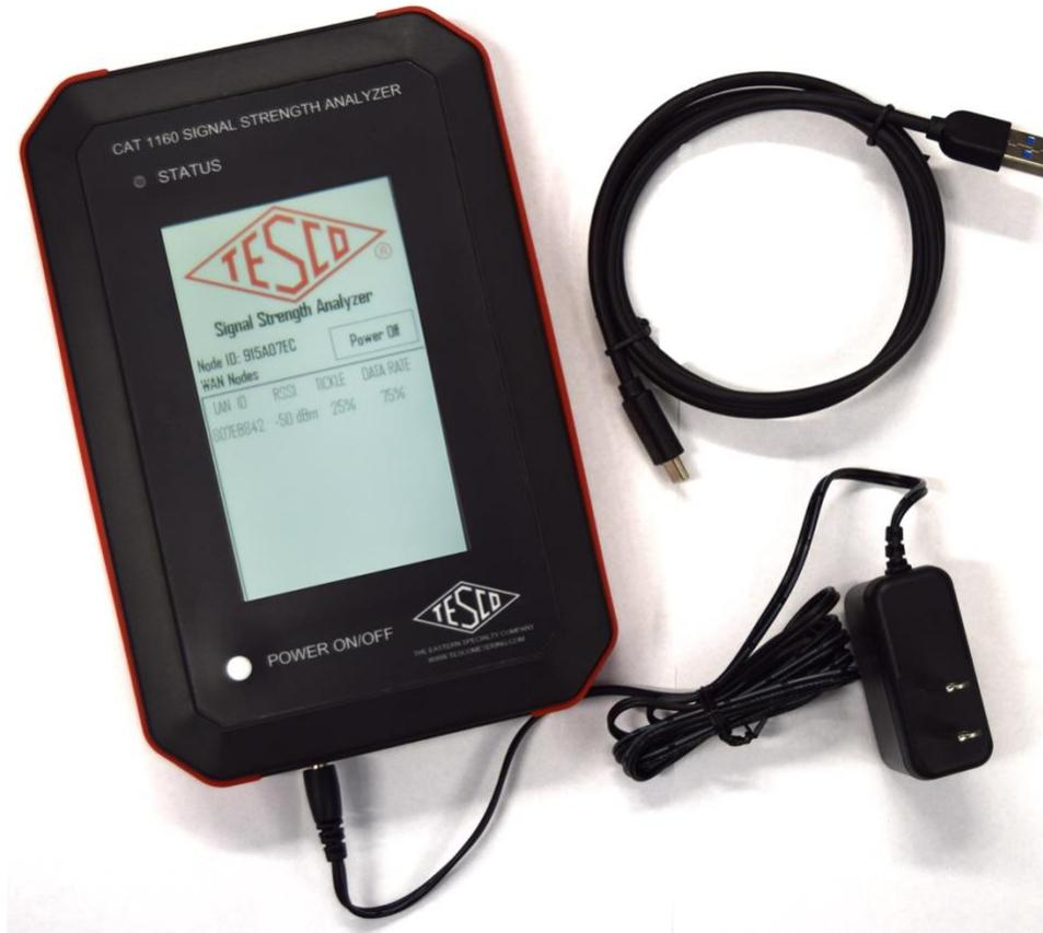
The Cat 1160, because of its new technology, requires that it be set up to join the customer's GridStream network. In order to do this, the customer must first connect the Cat 1160 to a computer that is running Landis + Gyr's RadioShop software, using the supplied USB-C to USB-A cable. The USB-C connector plugs into the port at the bottom of the Cat 1160.
