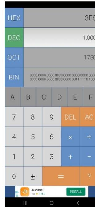
In our example, we will use 1000 as our Network ID. This equates to “3E8”. It should be noted here that both Offset values must contain two digits. If there are only 3 Hex digits in the address, fill in a leading 0 for “Offset 0”. In our case, “Offset 0” = 03, and “Offset 1” = E8. Enter these values into the “Value” field for each offset.
