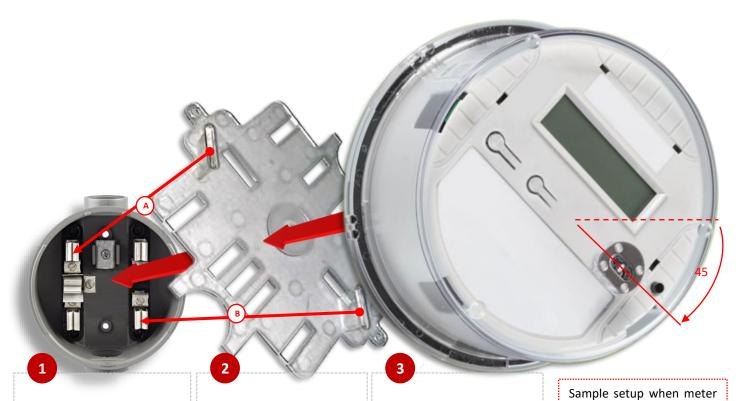
Locate and prepare meter socket where disconnect shield is to be inserted.
