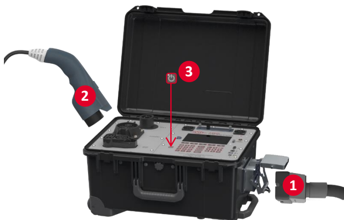
Figure 1.2 T4000 Connection and Power-Up
