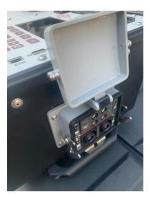
Put the Staubli connector of the PL4150 into the pins of the T4350. The bottom two circular connectors need to be facing in the downwards position.
