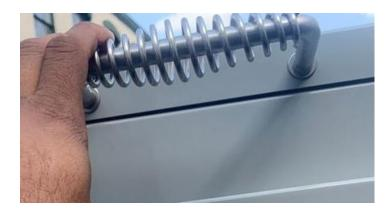
Relatch the two latches by hooking the metal latch to the top of the latch holder.
