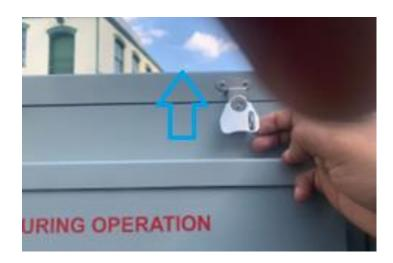
Twist the latch counterclockwise until it is completely undone.
