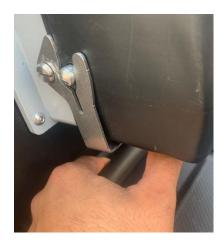
Fully remove the Staubli connector and return it to the PL4150. Ensure that the connector is tightly placed in the square bracket and lift the metal bar in the downwards position to lock it.
