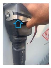
Unlock the Staubli connector of the T4350 by pushing down with force on the metal handle.
