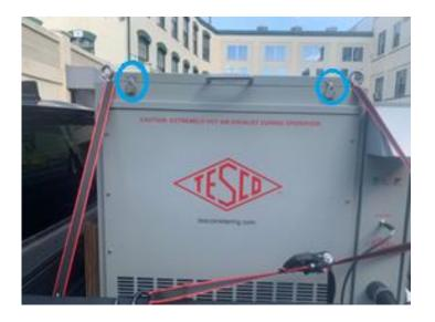
To unlatch, pop the bottom of the latch upwards.
