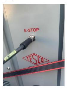
Before any transport, ensure the Staubli connector is properly secured to the L-bracket and the latch is down and tight so that it cannot move. This also ensures the connector is waterproof. The connector works by aligning the pins into the square and pushing the silver bracket down with force until it locks.
