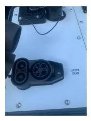
Lock your EVSE connector into the unit until you have it click and stay in place and begin the charge via the EV charger.
