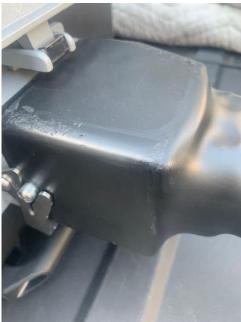
Push the bottom of the metal connector upwards with force until the connector is properly secured and it locks. The metal connector should be solidly in place and there should be no wiggle room in this connection.
