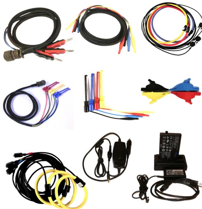
\*TESCO's Lightweight Kit pictured includes 6330 unit, B00-001 Battery Pack, 1037-SA Optical Pickup, CJO-6330-002 Current Jumpers, CCO-6330-002 Current Cable, VCO-6330-002 Voltage Cable, VTO-6330-001 Test Clips, and P01-0040-R Rogowski Current Probe. Total weight: 17.8 lbs.
