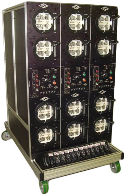
CUSTOM 3-PHASE QUALIFICATION BOARD
