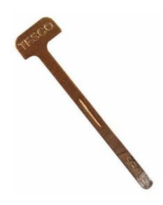
"T" SEALS CATALOG NO. 224 The TESCO "T" Seal is a locking device for electric meter covers. The "T" Seal can be easily installed and removed without any tools. The curved base is stamped "SEALED", and is scored to fracture if tampered with. The "T" Seals can be customized with up to five letters stamped on flag. Double-sided stamping is also available.
