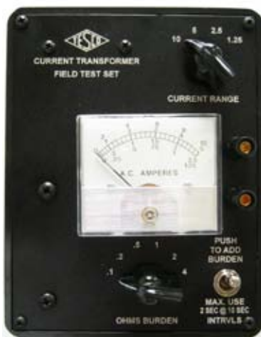
CURRENT TRANSFORMER BURDEN TEST SET CATALOG NO. 1043
